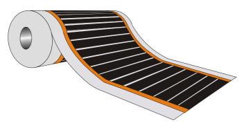
Although all Flexel element is visually inspected at the factory before dispatch, the elements should be checked to ensure any rough handling has not damaged the Flexel element. Look for creasing or folding that could have been caused by a roll of element being trodden on. Any such damaged areas must be discarded.
