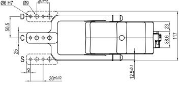
Min./Max. operating pressure: 0,4 / 0,8 MPa Operating temperature: 5° + 45° C Opening angle: adjustable from 0° to 135° Vertical arm mount position Electronic 24 Vdc sensor with M12 swivel connector that can be orientated at 0° or 90° Protection class: IP 65 Pneumatic ports on both sides
