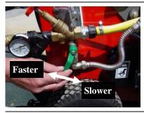
9) Adjust the speed of cart retraction by moving the bypass lever or speed control lever in the directions shown by the arrow. Closing this valve will increase retraction speed and opening the bypass valve will slow down the retraction speed
