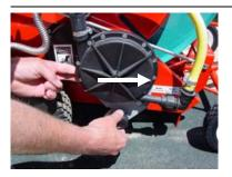
2) Loosen the black turbine lock knob as shown at the bottom of the image to the left by turning counter-clockwise. Now the turbine drive assembly and bracket will slide towards the sprinkler cart (as shown by white arrow) to disengage the turbine drive gears. Re-tighten the knob to hold the turbine drive gear away from the drum gear. Drum will now spin freely allowing sprinkler cart to be pulled out.
