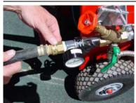
7) Attach supply hose provided to the inlet of the machine and lock into place as shown
