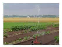
8) Turn on the water source to the MR25. The sprinkler equipped with the MR25 can be set to water a full circle pattern or any part of a circle. It is generally recommended to water a half circle pattern behind the cart, away from the direction of travel. The MR25 is equipped with a pressure regulator at the inlet to maintain system pressure at no more than 60 psi.
