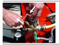
**6**) Open shut off valve by pulling the valve handle and latching into the open position by swinging the valve latch down and into position to hold valve open as shown.
