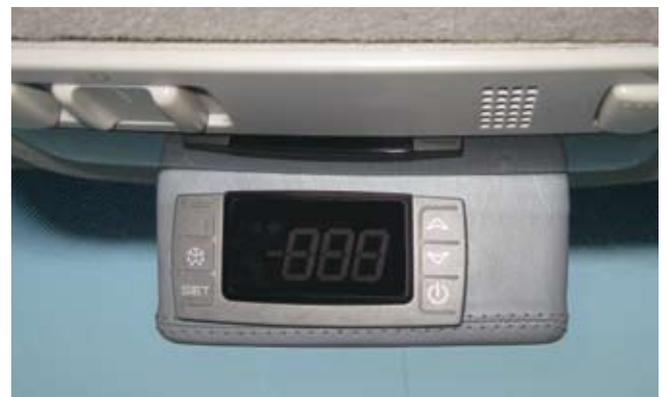
Neatly integrated: control element with vehicle-specific console (optional). The current cargo department temperature is always in view for the driver.
