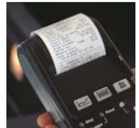
Real-time documentation: temperature logger + mini-printer + software
