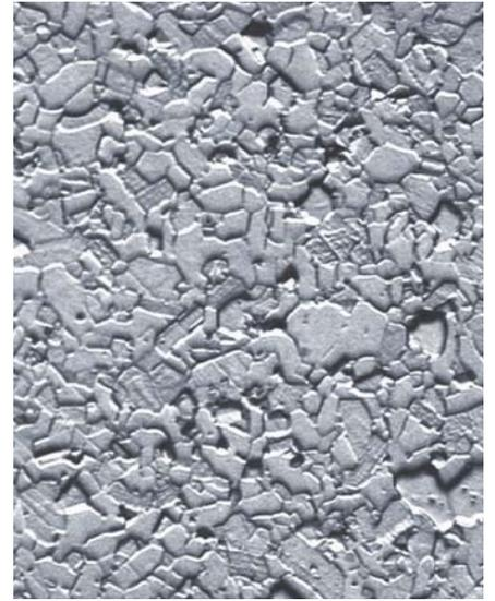
grain size < 5  $\mu\text{m}$ , density > 3.16  $\text{g}/\text{cm}^3$
