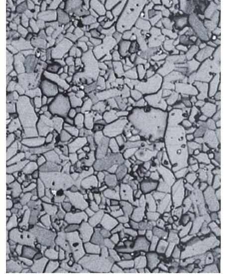
Mean grain size < 5  $\mu\text{m}$ , density > 3.10  $\text{g/cm}^3$
