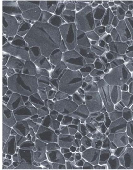
grain size < 2  $\mu\text{m}$ , density > 3.21  $\text{g}/\text{cm}^3$
