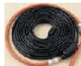
[EASYHEAT HB Series](#) Pipe Heating System. Keeps water flowing down to -40°F. Pre-assembled, ready to install. No thermostat, no plug. 7 watts per foot. 120 and 240 Volt AC and are suitable for use on plastic and metal water pipes. Cable is hard wired to the power source. 2 ft orange 14/3 cold lead.
