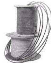
[Chromalox CWM](#) Constant Wattage Medium Temperature Heating Cable. Industrial/ Process and Commercial/ Construction. Flexible to Most Any Configuration. Fluoropolymer Jacket. 4, 8 and 12 W/Ft. 120, 208 - 277 and 480 Volt.
