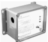
[ETI SST-2 Freeze Protection Thermostat](#) Automatic freeze protection, 40°F (4.4°C) set point, Automatic supply voltage selection. Two-pole contactor switches up to 30 AMP heater loads, Alarm relay with isolated contact, Integral 30 mA GFEP, C-UL-US listed, Simple to install and operate, Minimum energy costs
