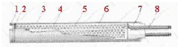
1. Heliarc welded end seal.
