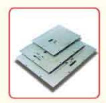
3. Heat Transfer Presses – Thin mica heater clamped to an aluminum plate is profiled to give very even temperature distribution. We achieved a 50% improvement in temperature distribution over the cast in tubular heater originally used. Performance increased and cost was reduced about 40%.
