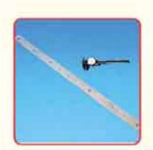
2. Sealing Bar – replaces expensive machined block bored for cartridge heaters. Mica heater is profiled for very even heat distribution (+-5F) across entire bar. The thin mica heater is sandwiched and bolted between two plates.
