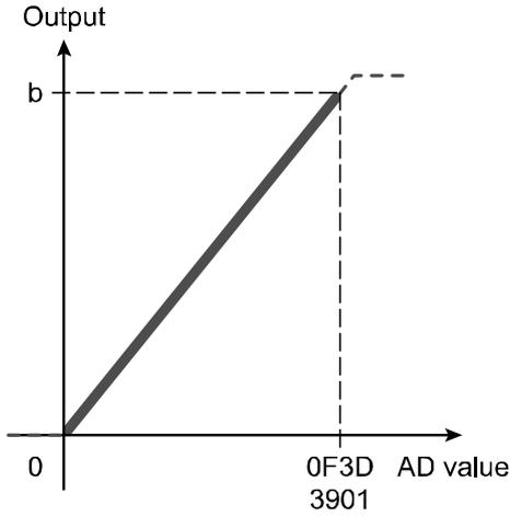
•Output signal range: 1 to 5 V, 4 to 20 mA
