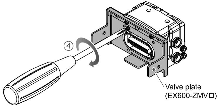
(5) Connect the SI unit and the valve manifold.
