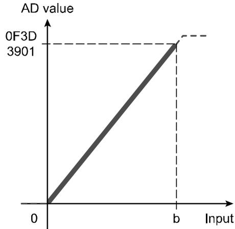
•Input signal range: 1 to 5 V, 4 to 20 mA
