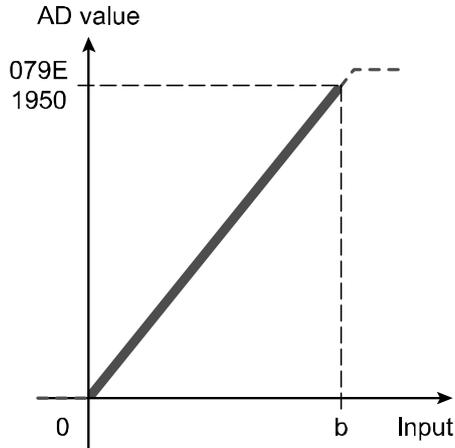
• Input signal range: 1 to 5 V, 4 to 20 mA
