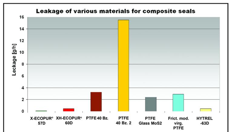
Fig. 12: Leakage of composite seals
