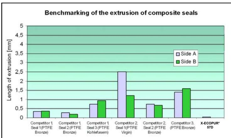
Fig. 18: Extrusion characteristics of commercially available composite seals compared to X-ECOPUR®-57D
