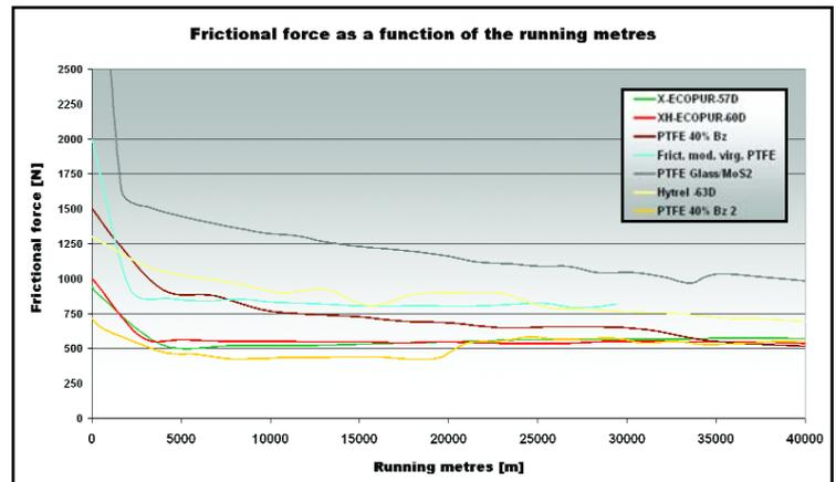
Fig. 11: Frictional force of various composite seals as a function of the running metres.
