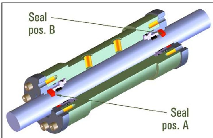
Fig. 4: Schematic drawing of the test cell
