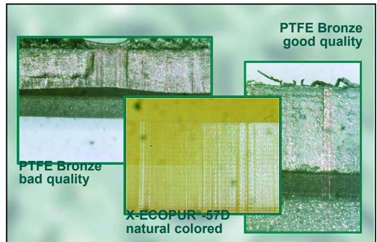
Fig. 15: Microscopic investigations of the sliding surface of composite seals
