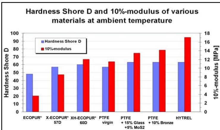
Fig. 7: Hardness and 10%-modulus of sealing materials
