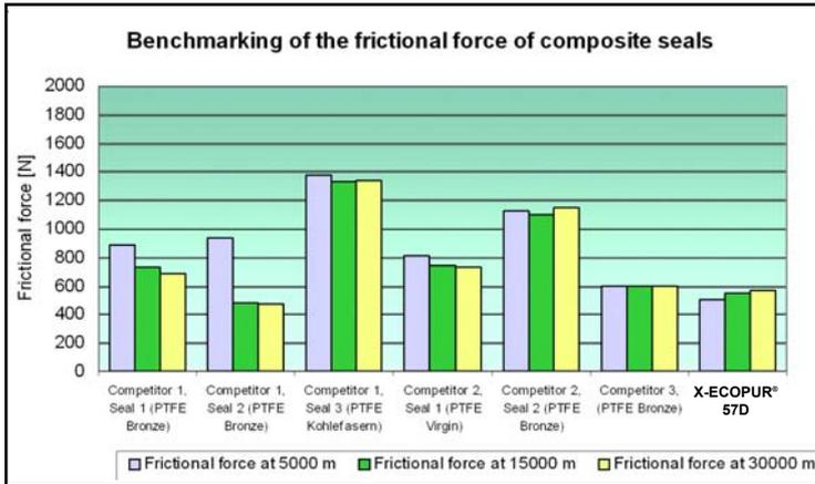
Fig. 16: Friction properties of commercially available composite seals compared to X-ECOPUR®-57D
