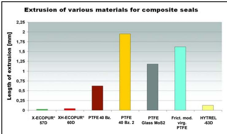
Fig. 13: Gap extrusion of composite seals
