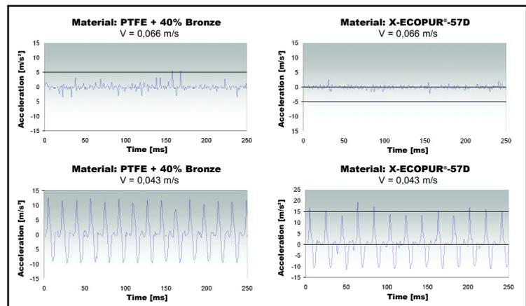
Fig. 19: Investigation of the stick-slip characteristics of composite seals
