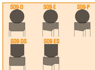
Fig. 2: Examples of co-axial and in-line composite seals for rod sealing
