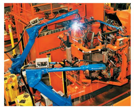
Fig. 3. The outer jacket of the "Roboflex recycle" lead, which is predominantly used in the body shells of car manufacturers, is not only resistant to welding beads but can also be recycled
