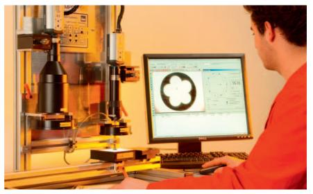
Fig. 2. Helukabel tests cables with the latest equipment in its own test center to determine whether the finished special cable and customer's sample actually comply with the characteristics required by the user
