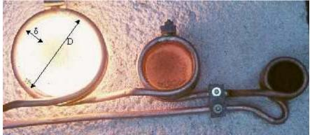
Three inductors are connected in line (equal current for every coil). The equation  $D > 2 \times \frac{1}{6}$  is only valid for the first coil (left side). The work piece in the last coil (right side) is not heated, because  $D < 2 \times \frac{1}{6}$ .
