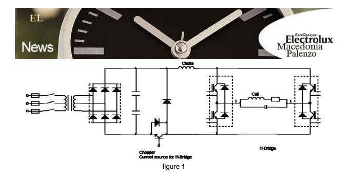
With the use of a mains transformer there is a potential-separation between the mains and the working circuit. Due to this design there is no short-circuit in case of an earth link at the induction-coil. The switching of the H-bridge is achieved with the switching of the chopper. Due to this solution it doesn't matter how often and under which power states the high frequency is switched on or off. There are no mechanical switches employed.
