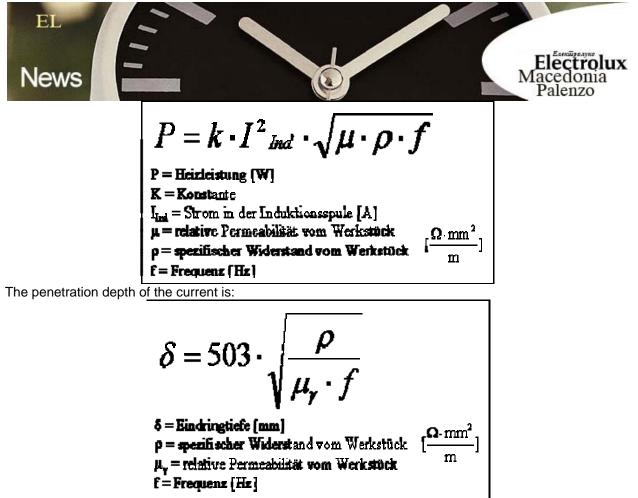
The formula is adapted to the case that the work piece diameter is at least double the penetration depth of the current.
