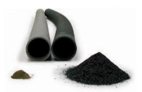
Visual differences in oxide spallation and sagging properties between the tube Kanthal APMT (left) and a standard Fe-Ni-Cr tube after 2 300 h at 1 100°C (2010°F).
