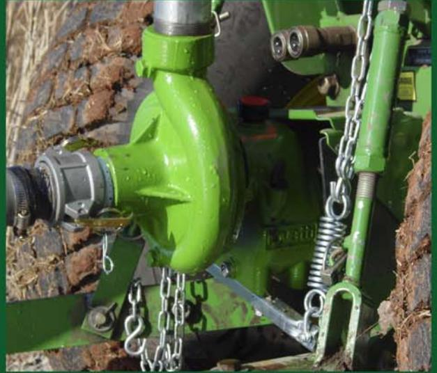
Rovatti T0F50 pumps are an extremely easy, portable, user friendly pump which can be directly attached to the PTO of most any 540 RPM tractor. Whether to fill ponds, sprinkler irrigate, wash down, transfer or tank filling, the T0F50 provides the solution inexpensively. The pumps provide up to 150 GPM and pressure as high as 75 PSI. The units come standard with a foot valve, suction and discharge fitting. These units are available in either standard centrifugal or self priming models.
