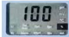
At the end of the calibration phase, the instrument indicates the state of efficiency of the electrode with a per cent value.
