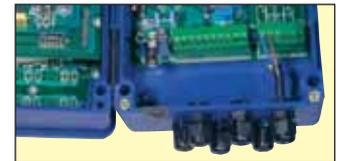
The instruments enclosure are protected in order to allow the use in industrial environments, thanks to the sturdy container that protects both the cabling connectors and the connection of the electrode.
