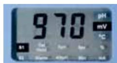
The instrument uses a LCD display with high contrast with characters of 15mm. An important characteristic of the display is the possibility of visualizing, without any alteration, at temperatures from -20 to +70°C. The flashing backlighting indicates the alarm state making it visible in any application condition.
