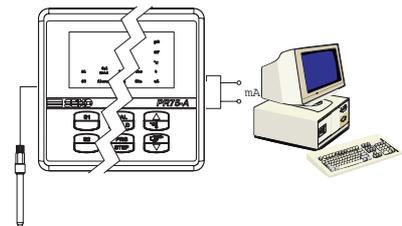
The galvanic separation of the output 4-20 mA is the ideal solution in order to avoid interference when you have to connect with a data acquisition system, PLC or recorder. It is supplied, on request, on the whole range.
