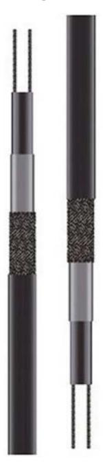
Self-regulating heating tapes consist of two parallel buswires, embedded semi-conductive self-regulating matrix. This means that the heating cable automatically responds to changes in ambient conditions.
