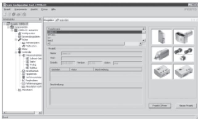
The main requirements for product configuration software are speed, reliability and user-friendliness. The multi-axis controller CMXR, like other products from Festo, is configured via the Festo Configuration Tool (FCT). Electrical variables (e.g. inputs and
