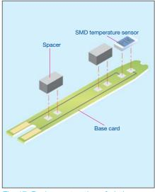
Fig. 17: Basic construction of platinumchip temperature sensors on epoxy card (PCSE style)
