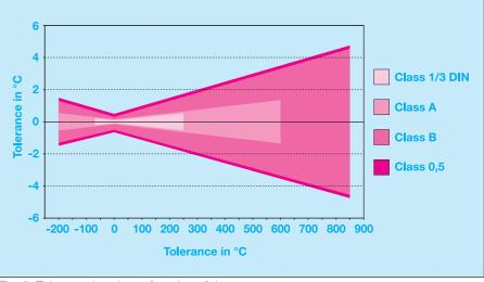
Fig. 2: Tolerance band as a function of the temperature
