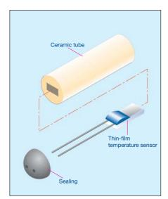
Fig. 15: Basic construction of platinumchip temperature sensors in cylindrical form (PCR style)
