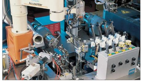
Fig. 9: Automated production of wirewound platinum-glass temperature sensors
