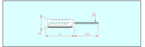
Dim. tolerances:  $\Delta D = \pm 0.3 / \Delta L = \pm 1.0 / \Delta D1 = \pm 0.02 / \Delta L1 = \pm 1.0/-2.0$ ; with 2 x Pt100 ±5.0
