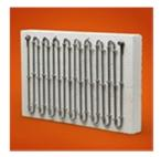
Prefabricated heating modules with metallic heating elements and non-electrically conductive, dense ceramic insulation for use at element temperatures up to 1350°C (2460°F).
