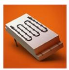
Prefabricated heating modules consisting of vacuum-formed ceramic fibre with an integral Kanthal Super molybdenum-disilicide (MoSi2) heating element for up to 1750°C (3180°F) element temperature.
