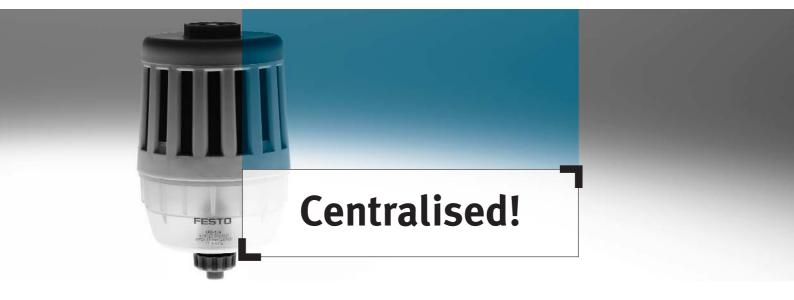
The filter silencer cleans all exhaust air from pneumatic control systems and reduces exhaust noise. Condensate is collected in the lower plastic bowl and is discharged via the condensate drain.
