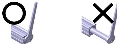
12. **When rotational torque is applied to the plate end, use within the allowable range. [LEYG series]**
