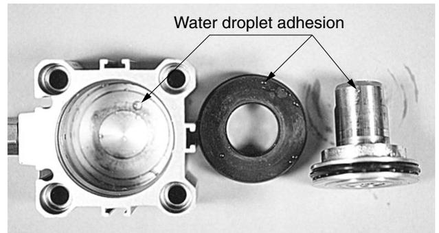
Photo 2 Dripping of condensation in a cylinder
