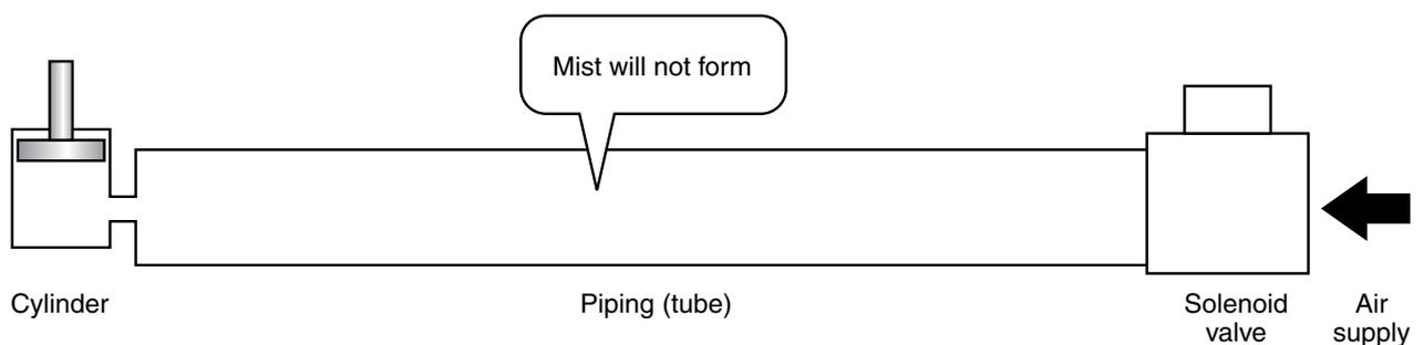
Note) Most piping is usually long, with a larger volume than the cylinder volume. Therefore, the piping is larger than the cylinder in the above figure.
