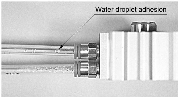
Photo 1 Condensation inside tube
