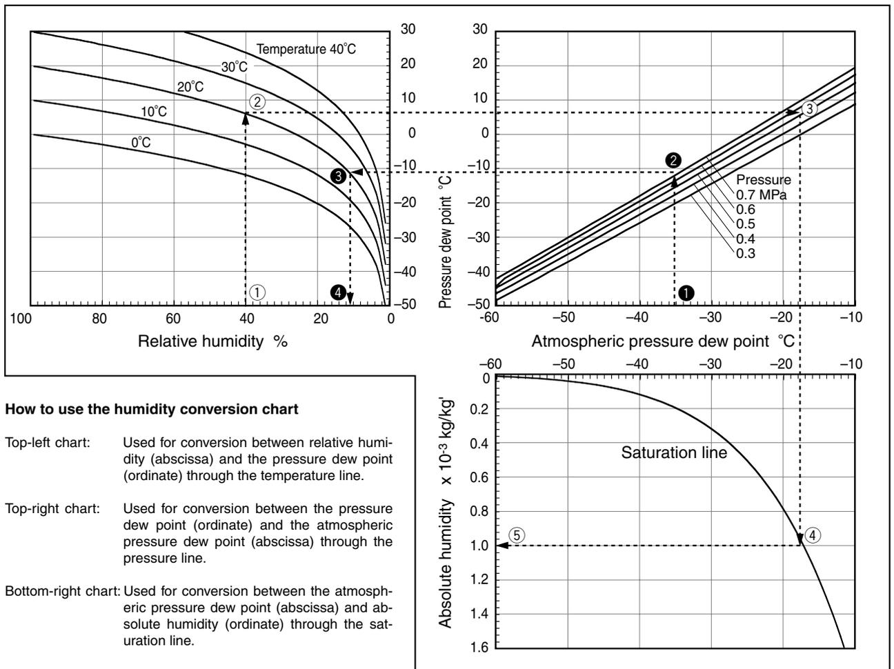
[Example 1] The absolute humidity of compressed air of 0.5 MPa pressure, 20°C temperature and 40% relative humidity is found to be 0.001 p<sub>kg</sub>/ kg' through the steps ①→②→③→④→⑤.
