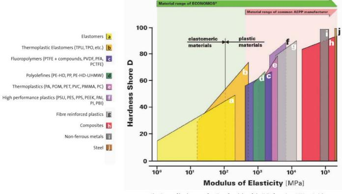
Fig.: Range of hardness as a function of modulus of elasticity for various AEPP material groups
