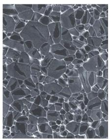
grain size  $< 2 \mu m$ , density  $> 3.21 \text{ g/cm}^{\text{s}}$
