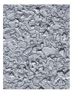
grain size < 5 µm, density > 3.16 g/cm<sup>3</sup>
