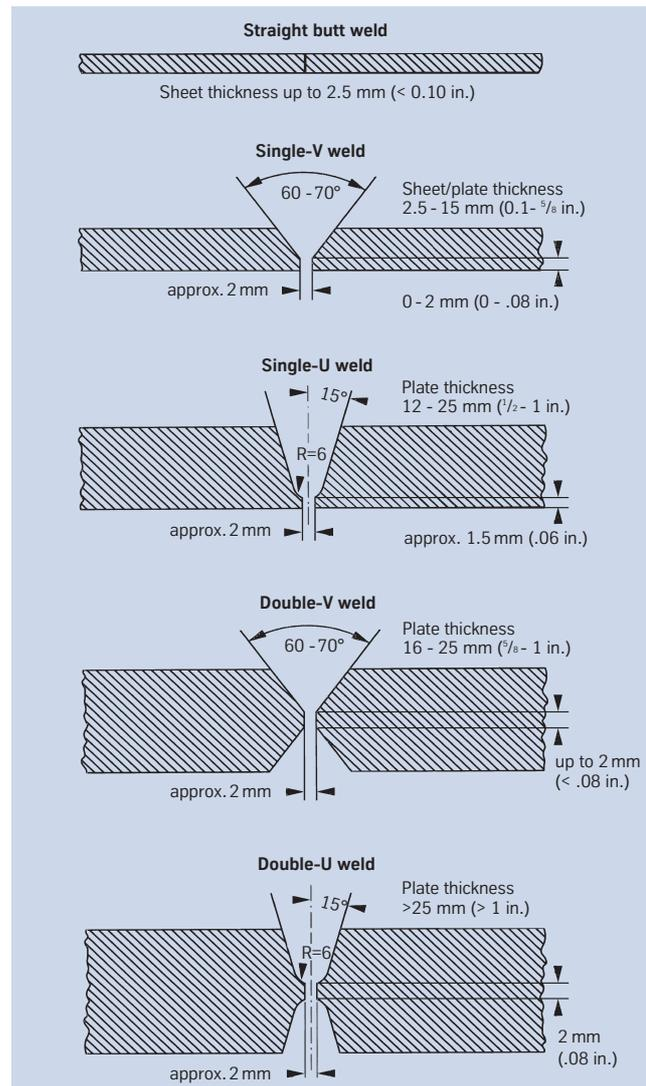
Fig. 11 – Edge preparation for welding of nickel alloys and special stainless steels.
