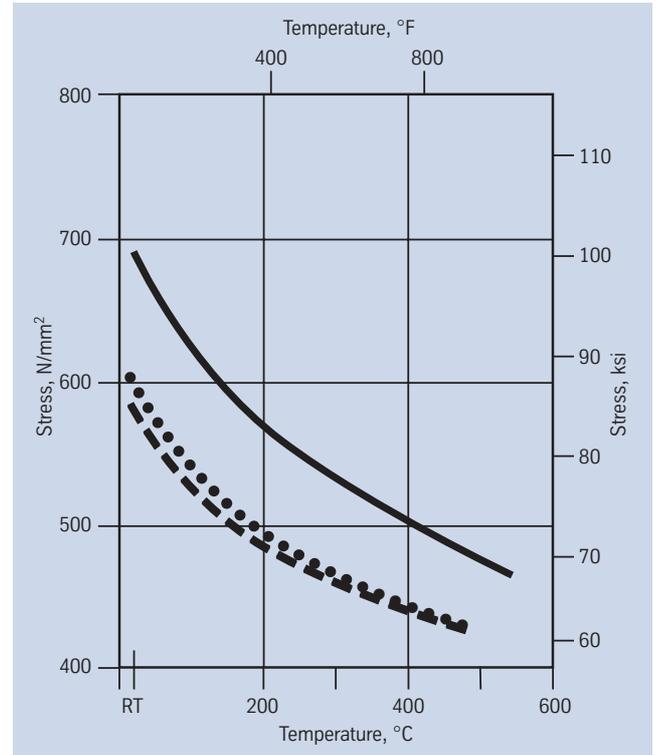
Fig. 2 – Typical short-time tensile strength at room and elevated temperatures.
