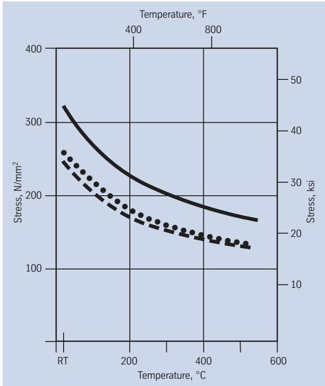
Fig. 1 – Typical short-time 0.2% yield strength at room and elevated temperatures.
