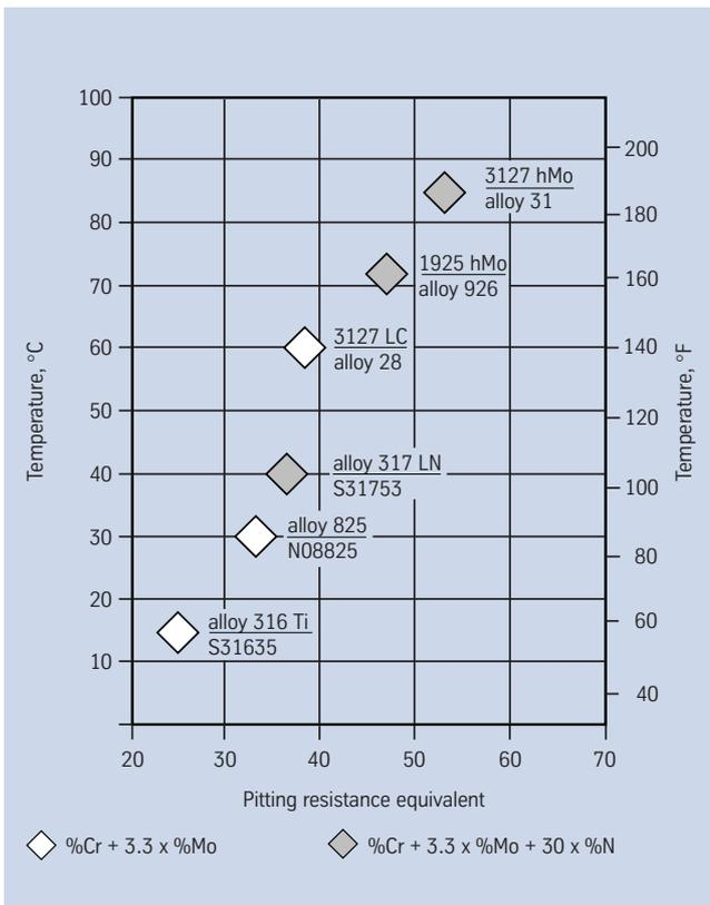
Fig. 6 – Critical pitting temperatures (CPT) in 10% FeCl<sub>3</sub> x 6H<sub>2</sub>O solution as a function of the respective pitting resistance equivalents (PRE).
