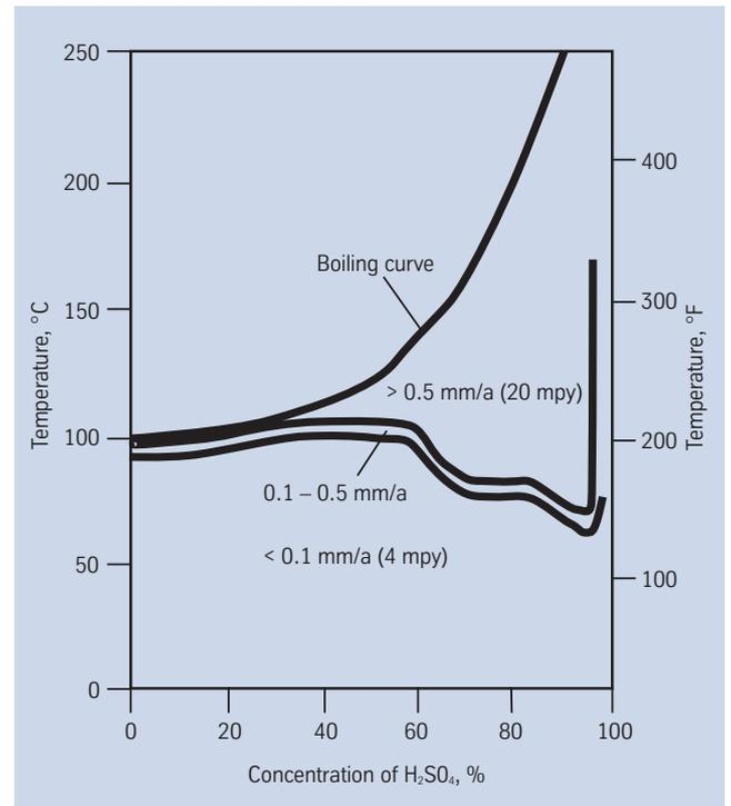
Fig. 3 – ISO-corrosion diagram of Nicrofer 3127 hMo in lightly aerated, technical grade sulfuric acid based on immersion test results over at least 120 h.
