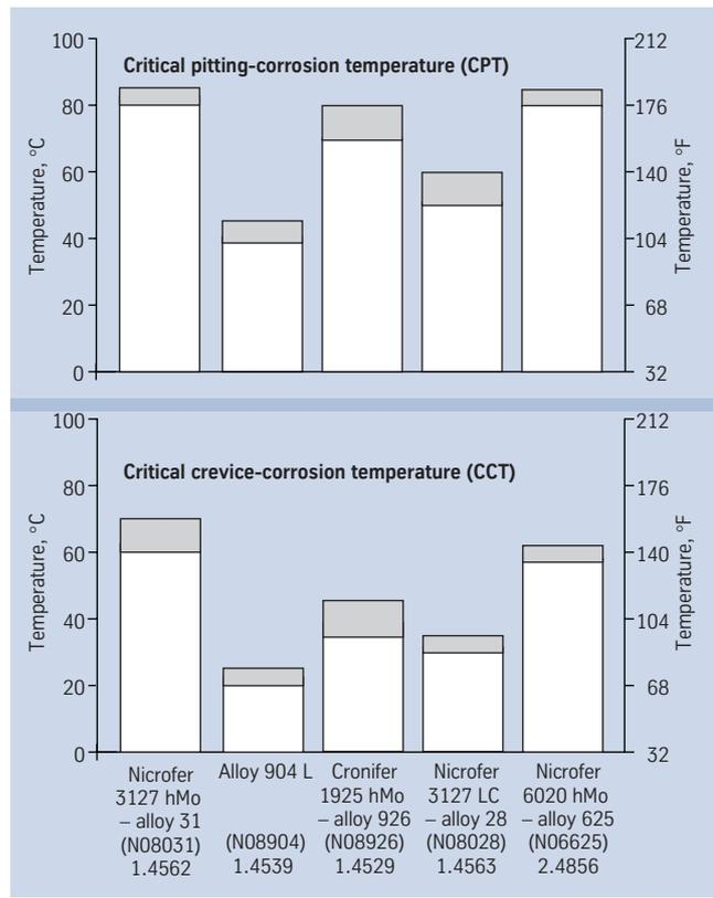
Fig. 7 – Critical pitting and crevice-corrosion temperatures of different alloys in 10% FeCl<sub>3</sub> x 6H<sub>2</sub>O solution.
