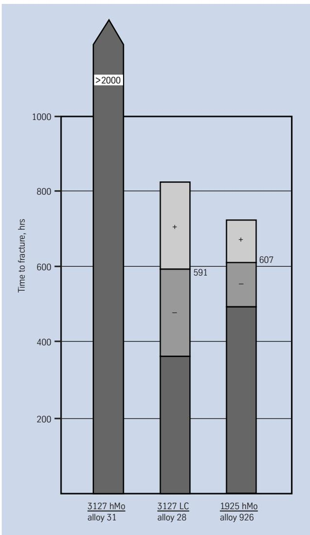
Fig. 10 – Stress corrosion cracking test with U-bend specimens in boiling 62 % CaCl<sub>2</sub>-solution.
