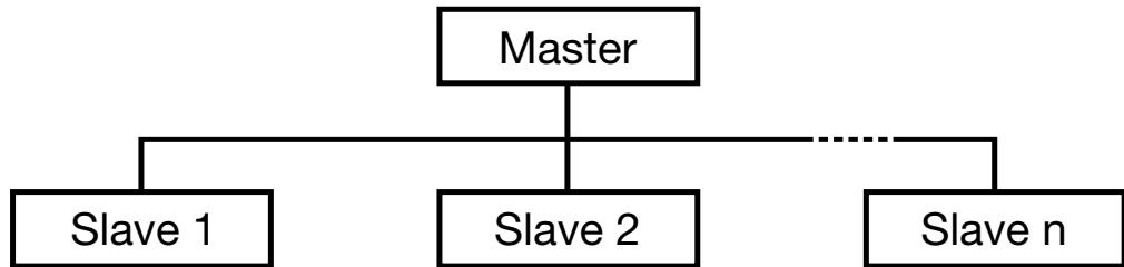
The master controls the data exchange, the slaves only have a response function. They are identified by their device address. A maximum of 255 slaves can be addressed.
