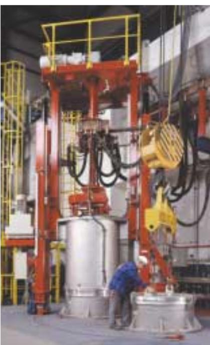
All ThyssenKrupp VDM alloys have their origin in the company's ultra-modern melting plant at Unna near Dortmund. The Unna plant is equipped for the melting and ladle treatment of high-nickel superalloys, high-alloy special stainless steels and copper-nickel alloys. The sizes and arrangement of buildings, furnaces and materials handling facilities were designed for maximum efficiency in material flow and easy enlargement.
