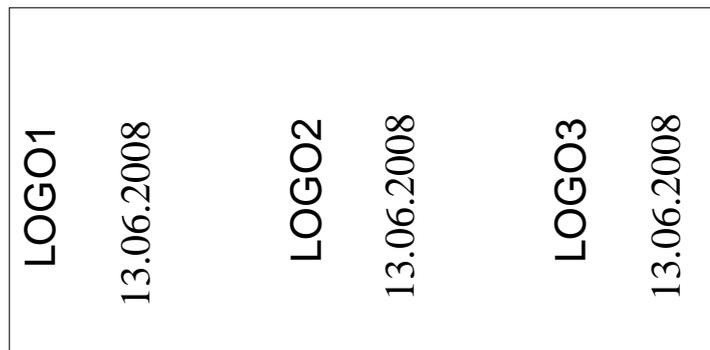
Supposed that the print speed is so high that no field ribbon save is possible, but after a lane enough time is available then by means of the shift ribbon save the gap of the fields can be filled with suitable layouts
