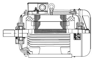
Frame size 280/4-6-8...355 D-End: Roller Bearing 9 N-End: Fixed Ball-Bearing
