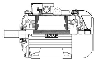
Frame size 63...132 D-End: Floating Ball Bearing (Spring-loaded) N-End: Floating Ball-Bearing
