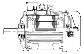
Frame size 160...280/2 D-End: Floating Ball Bearing (Spring-loaded) N-End: Fixed Ball-Bearing
