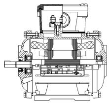
Frame size 56 D-End: Floating Ball Bearing (Spring-loaded) N-End: Floating Ball-Bearing
